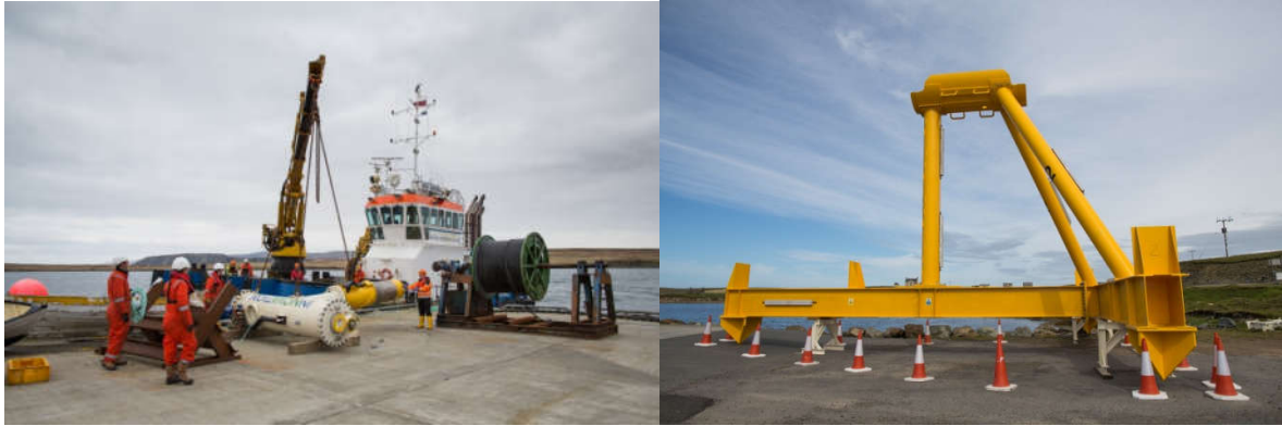
Nova Innovation's 30kW tidal stream turbine deployed in 2014 and the base of the first 100kW machine now being deployed in September 2015.
